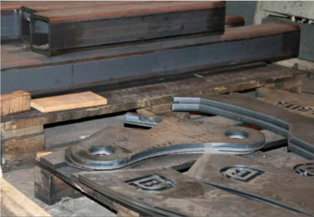
Steel profiles, and pre-cut hollow sections, ready for fabrication.
