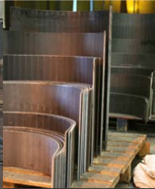
Pre-bent, bucket back plates, formed in-house on our CNC press brake,.
